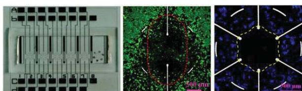
A microfabricated cell-based electrochemotherapy (ECT) testing device which mimics a clinical electroporator of circular needle-array is demonstrated to study the electrochemotherapeutic effect on T47D human breast cancer cells. Until now, the performance between electroporators having two- and six-needle circular array
