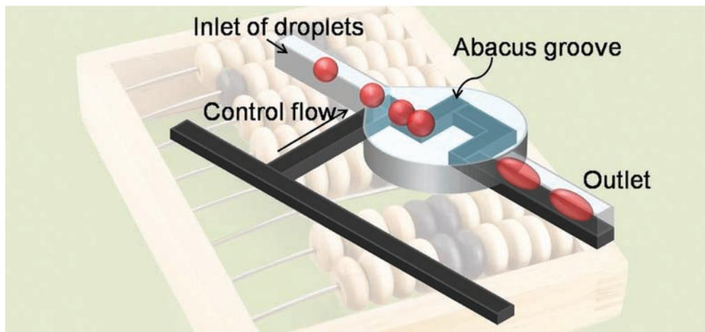
Korean scientists have created a microfluidic abacus that allows them to add droplets together. The system can mimic the logic operations of an electronic chip, they say.
