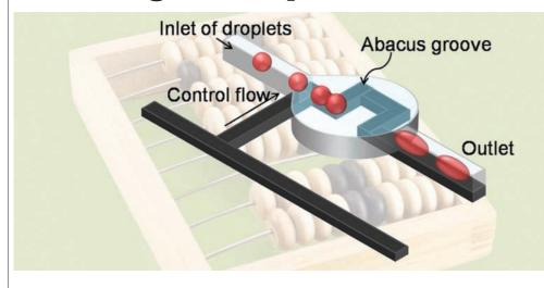
Korean scientists have created a microfluidic abacus that allows them to add droplets together. The system can mimic the logic operations of an electronic chip, they say.
